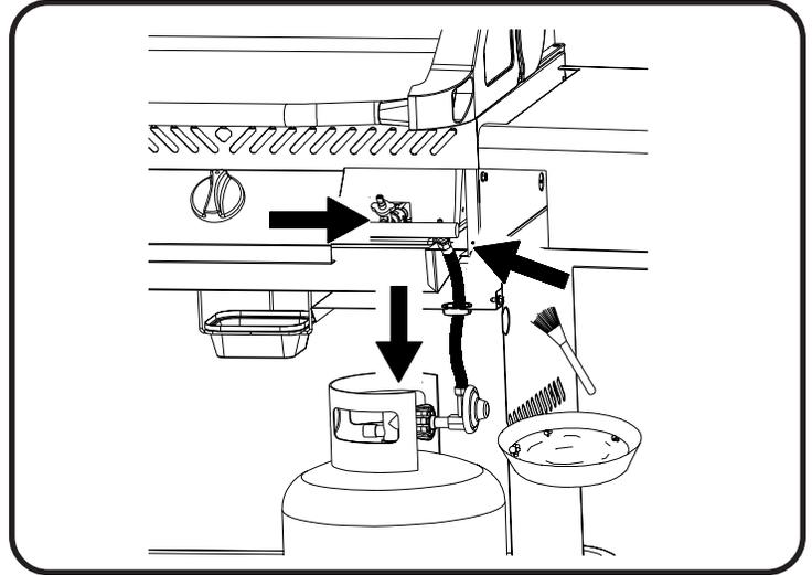
**LEAK TESTING:** This must be done before initial use, annually and whenever any gas components are replaced or serviced. Do not smoke while performing this test, and remove all sources of ignition. See *Leak Testing Diagram* for areas to check.
